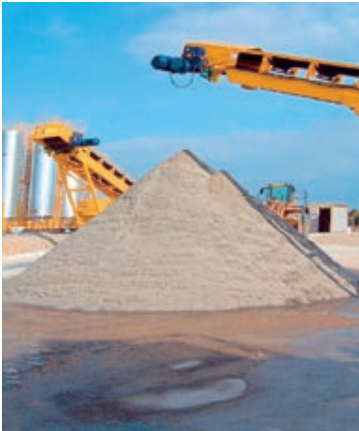
More than 20,000 tonnes of pretreated sludge (limed and pressed) were fed into the kiln lines of Holcim France-Benelux.
