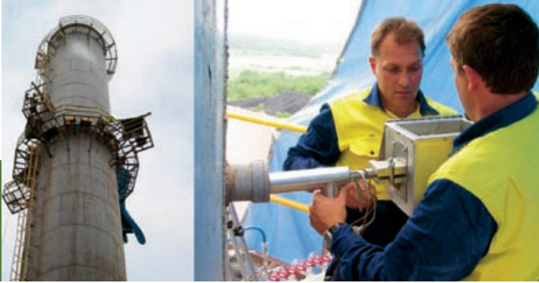
Stack with the monitoring platform and the adjustment of the probe into the kiln
