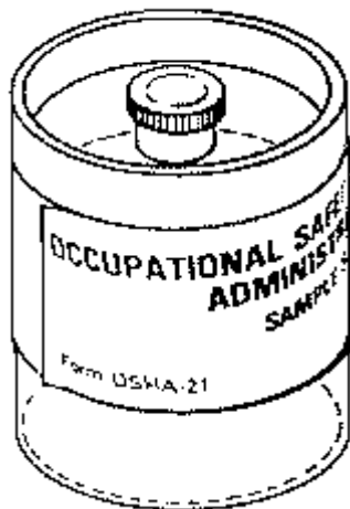
FIGURE II:1-1b. IMPROPERLY SEALED CASSETTE ALLOWS ACCESS TO INLET AND OUTLET AFTER SAMPLE HAS BEEN TAKEN.
