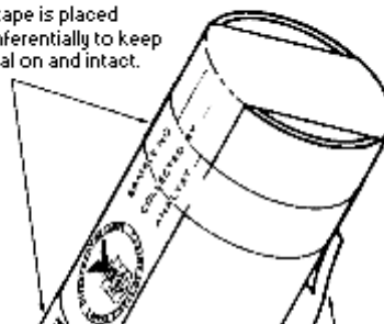
FIGURE II:7. A STANDARD ASBESTOS CASSETTE (25 mm) SEALED PROPERLY WITH AN OSHA 21 FORM
